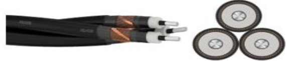
POLYCAB MV AL BS 7870-4-10 12.7/22 KV Triplex - Medium Voltage Copper wire screened Cable, 12.7/22 (24) KV AC
