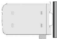
Fig. 3 Top-hat rail Mounting
