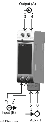
Fig. 6. Front View of Device for electrical Connections
